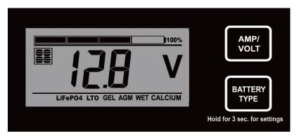
Press **BATTERY TYPE button** and hold for 3 seconds to go into your battery type selection mode, the battery types you select will be shown on the LCD meter, the default setting is AGM Battery; the controller will automatically memorize your battery type setting.
