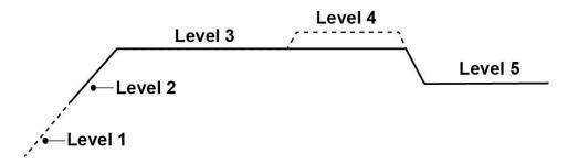
**Soft Charge**- When batteries suffer an over-discharge, the controller will softly ramp the battery voltage up to 10V for 12V battery, 20V for 24V battery.
